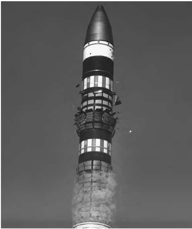
Shock-absorbing pads fall away from the surface of an LGM-118A Peacekeeper intercontinental ballistic missile as it emerges from its launch canister. This photograph is from the first test launch of the Peacekeeper, on 17 June 1983 at Vandenberg Air Force Base, California. (U.S. Department of Defense)
