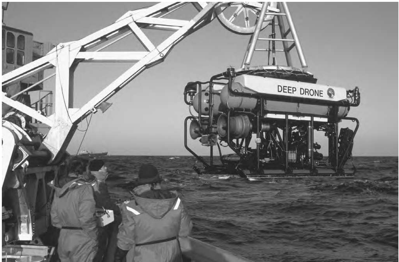
The U.S. Navy submersible Deep Drone being readied for deployment from the U.S. Navy fleet tug Narragansett during the search for Korean Airlines Flight 007, 1 July 1984. (U.S. Department of Defense)
