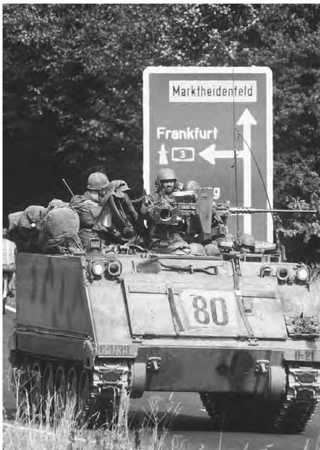
A. U.S. Army M-113 armored personnel carrier mounting a 12.7mm machine gun passing a German road sign during the multinational NATO exercise REFORGER 82. (Department of Defense)
