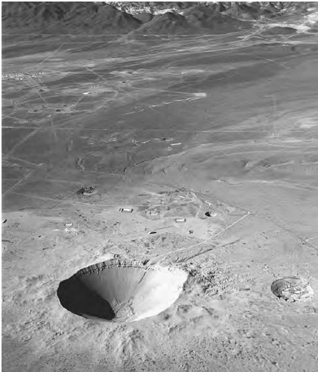
Crater at the Nevada Test Site in Mercury, Nevada. It was formed when a 100 kiloton explosive buried under 635 feet of desert alluvium was fired at the site on 6 July 1962. The crater is 320 feet deep and 1,280 feet in diameter. (U.S. Department of Energy)
