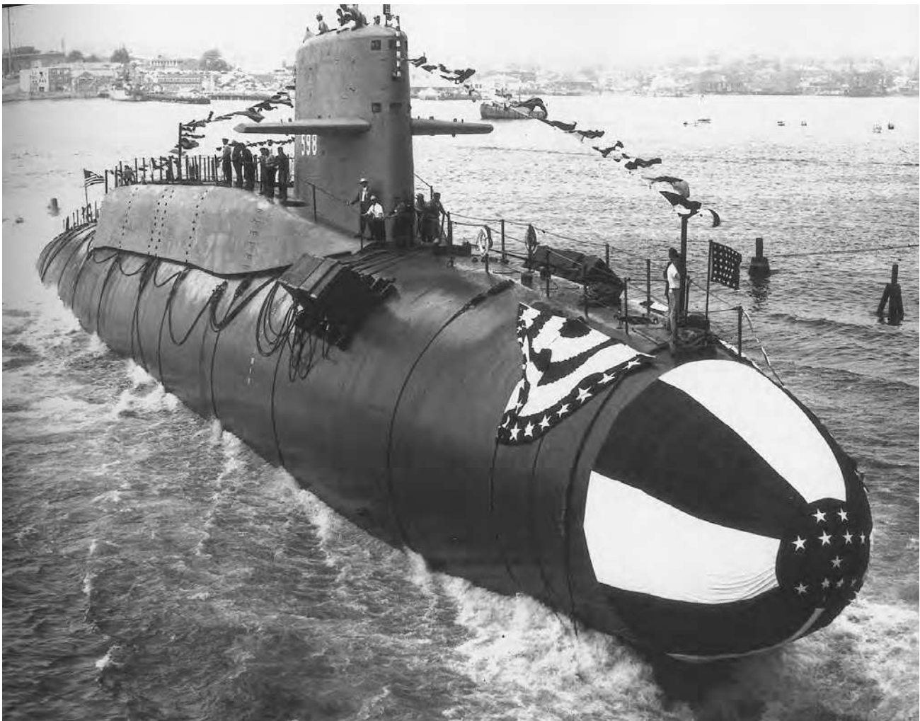
United States Navy ballistic submarine George Washington , the first nuclear-powered submarine designed to launch Polaris ballistic missiles while submerged, on its launching at Groton, Connecticut, 9 June 1959. The George Washington was built quickly by cutting an attack submarine in half and adding a missile compartment. (United States Naval Institute)
