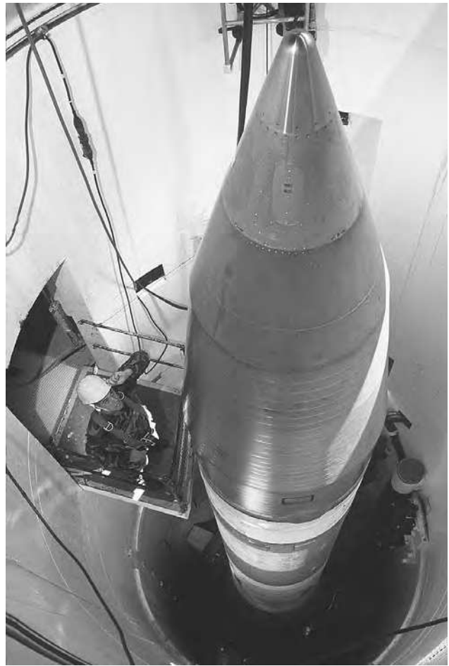
Inspection of an LGM-30G Minuteman III missile inside a silo about 60 miles from Grand Forks Air Force Base, North Dakota, 1989. (U.S. Department of Defense)
