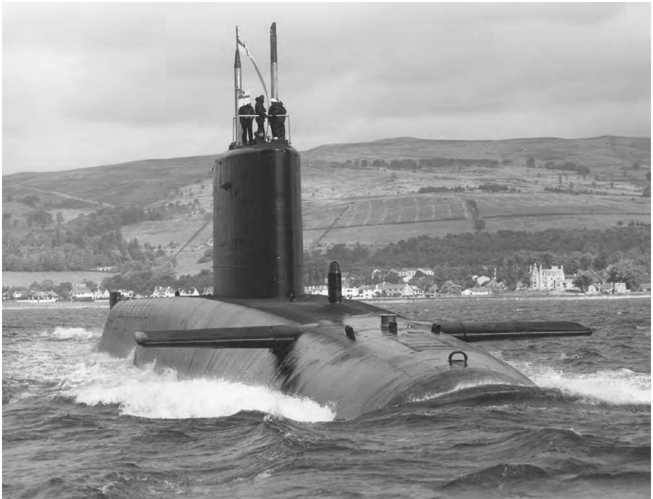
Royal Navy Resolution-class submarine, 1966. The Resolution-class were the first British strategic ballistic missile submarines and carried the Polaris missile. (Art-Tech)
