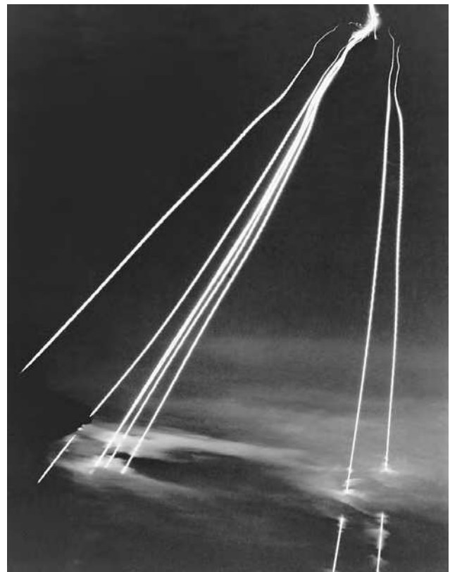
A time exposure of eight Peacekeeper (LGM-118A) intercontinental ballistic missile reentry vehicles passing through clouds while approaching an open-ocean impact zone during a flight test, 20 December 1983. (Department of Defense)
