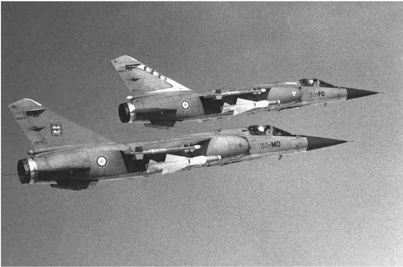
Two French Air Force Dassault Mirage F-1C aircraft armed with Matra 550 Magic air-to-air missiles on the wing tips and Matra R.530 air-to-air missiles under the fuselage, May 1986. (U.S. Department of Defense)
